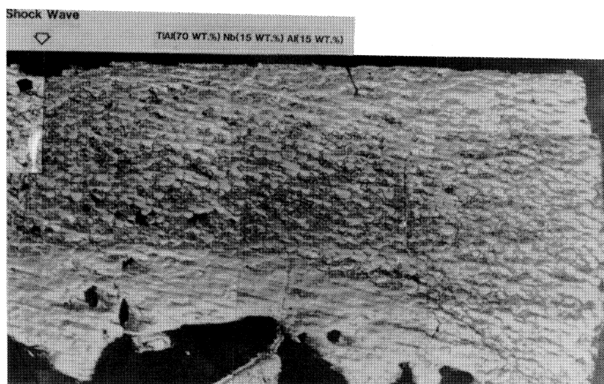
FIG. 9. Micrograph of cross section of compact containing a mixture of 70 wt. % TiAl, 15 wt. % Nb, and 15 wt. % Al powders after passage of shock wave (2.3 km/s impact velocity). Bottom figure shows microhardness measurements in various parts of the compact.
